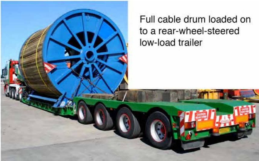
Figure 39 – Cable drum loaded transversely onto a trailer
