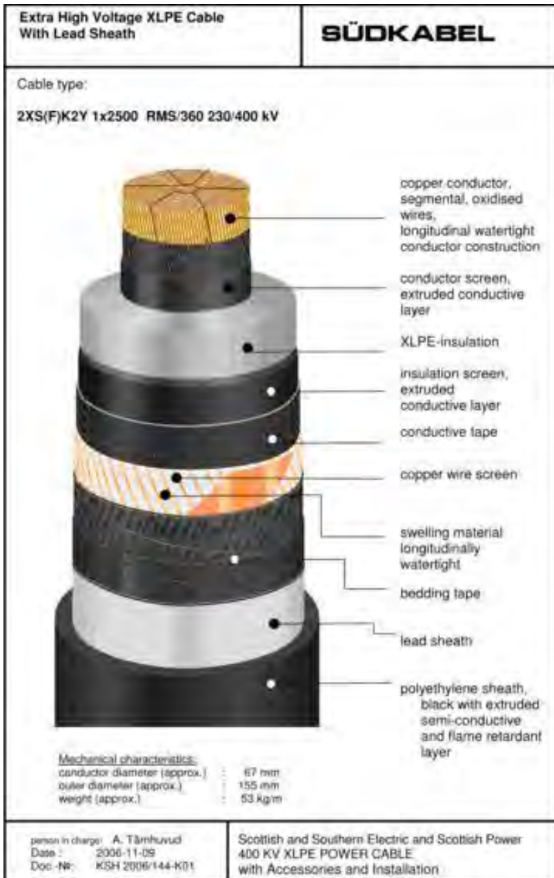
Figure 18 – Diagram of a 400kV transmission power cable
